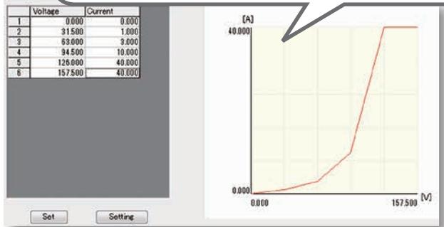
[Direct control window] Directly control PLZ-5W in a manner similar to using a remote control. In addition, monitoring and logging of output are also possible.
