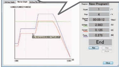
[Arbitrary I-V characteristics (ARB) mode] In the arbitrary I-V characteristics (ARB) mode, desired I-V characteristics can be set by specifying multiple arbitrary points of I-V characteristics (as sets of voltage and current values).
