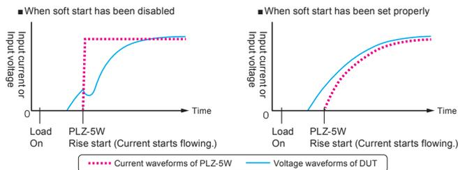
Can be set to OFF / 100 μs / 200 μs / 500 μs / 1 ms / 2 ms / 5 ms / 10 ms / 20 ms. This sets the soft start time.
