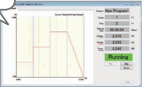
[Monitor graph] Current values for current, voltage, and power can be checked for the sequence being executed on a graph in real time. Monitor data is displayed by placing the mouse cursor on the graph.
