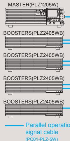
Parallel operation using the same type of electronic loads
